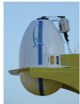
Figure 7. A close-up of the Vindicator unit which is mounted on the buoy (Fig 6) and measures wind speeds at multiple heights using laser pulses.
