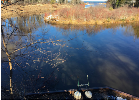
A DIDSON unit was deployed at Bell Landing near the Ocqueoc River mouth in Presque Isle County. The camera is submerged and mounted to the steel seawall at the bottom center of the photo. Photo: Erin McCann
