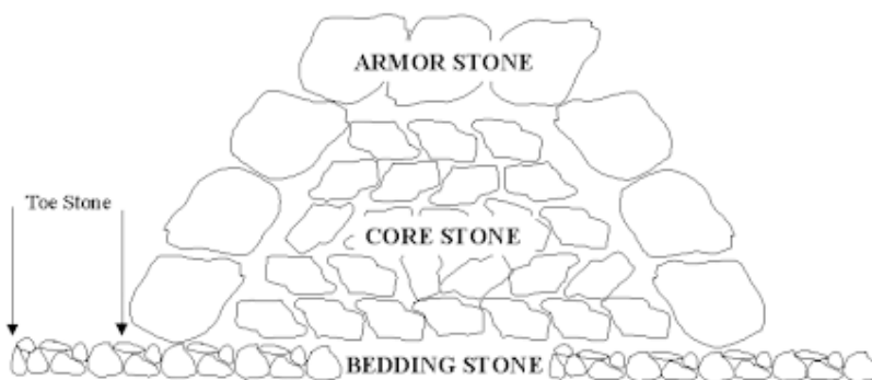
Figure 7 Typical cross-section of a rubble mound breakwater.
