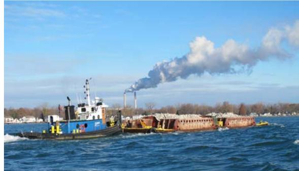
A side-dump barge used to drop rock
