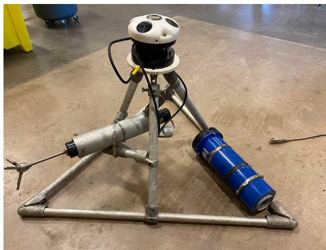
Underwater, self-recording instruments are being used to monitor how storm-induced waves move sediment from the nearshore to deep water where it is lost from the beach forever. Photo: Guy Meadows
