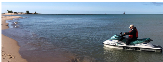
The research team developed a novel technique for mapping onshore and offshore changes using a jet ski to rapidly measure changes in the underwater portion of the beach in response to severe storms and water level changes. Photo: Guy Meadows
