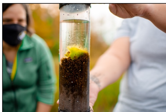
Figure 4. Image of core taken from a microcosm in the Nara Nature Preserve for in lab flow through incubation experiments. Photo Credit: Sarah Atkinson at Michigan Technological
